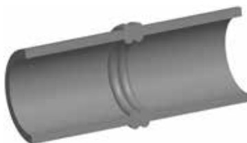
Figure C.3: Bead design at heated tool butt welding (principle) of a pipe.
