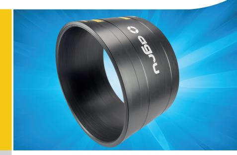
The new AGRU E-coupler machined in completes the system and opens new application fields. Leightweight and thus easy to handle, the E-coupler made from PE 100-RC requires short welding times. Ovalities of the components to be welded as well as big annular gaps are compensated widely to provide a perfect welding result. If for sewage, industrial applications or fishfarming, the AGRU E-coupler provides the perfect fit.
