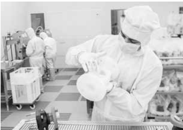
Figure B.7: Cleanroom valve testing and assembly
