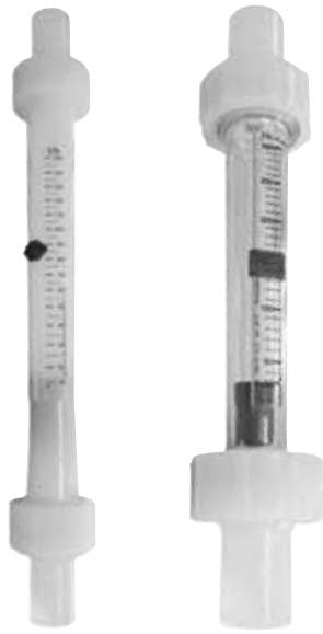
Figure G.94: Flow meter.
