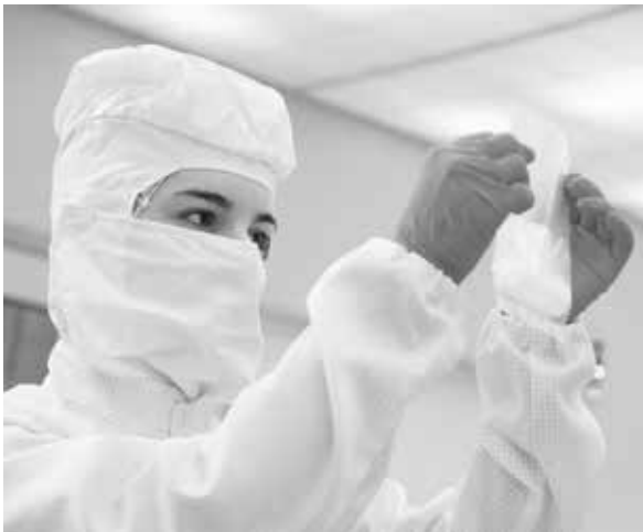
Figure B.9: Cleanroom packaging of fittings/valves.
