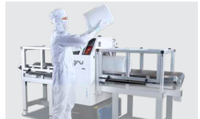
CleanCut 315 cutting machine for precise pipe processing in cleanroom quality
