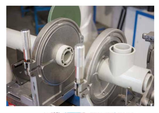
The AGRUCHEM Poly-Flo double containment piping system can be joined using time-saving simultaneous welding.
