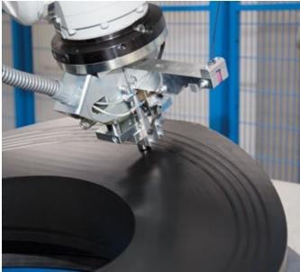
CNC production machine for heating wire insertion
