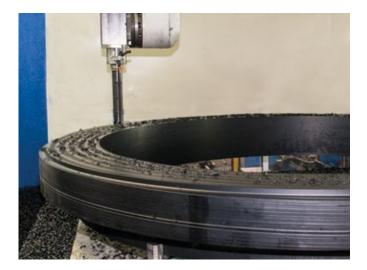
**3 and 5-axis CNC milling machines** Round parts up to 2600 mm diameter. Maximum travel distance 3000 x 2600 x 2000 mm.
