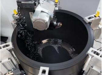
**CNC turning machines** Round parts up to 1600 mm diameter. Maximum travel distance 1700 x 700 mm.
